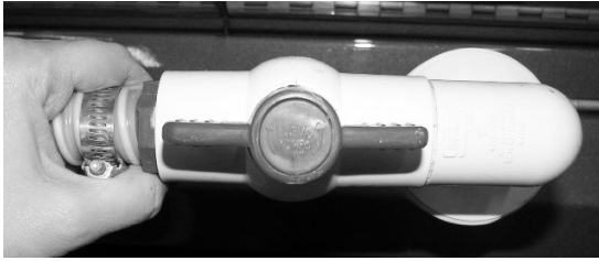
Sewage Drain Hose Valve
