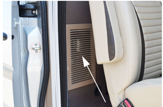
Water Pump (Located behind removable vent on front side of shower cabinet)
