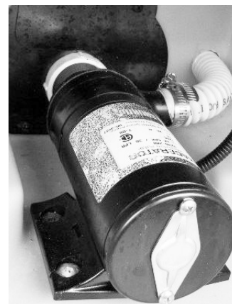
Waste Pump (Located beneath coach) -Typical View
