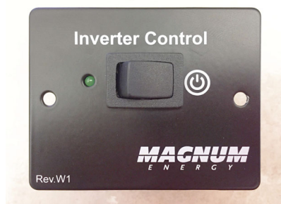
Inverter Control Panel (Located near monitor panel) -Typical View
