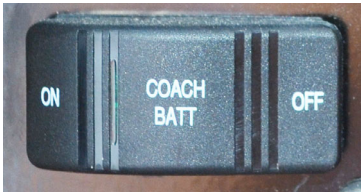
House/Coach Battery Disconnect Switch
